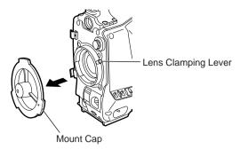
Align the indentation at the top center of the lens mount with the center mark of the lens and mount the lens.
